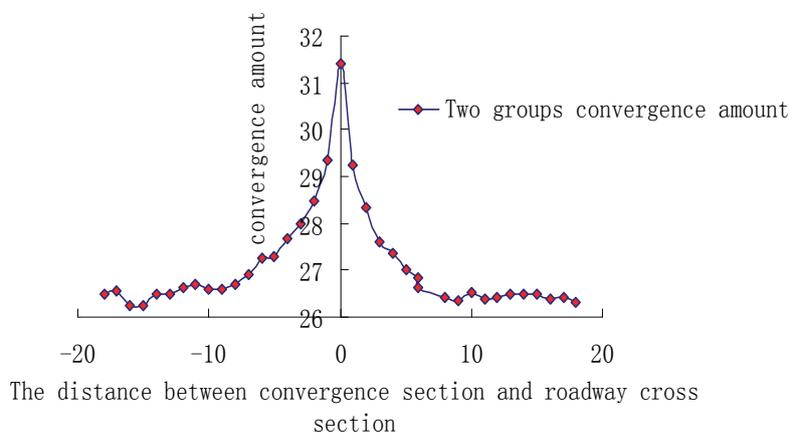
Figure 9 The main roadway transverse displacement curve
