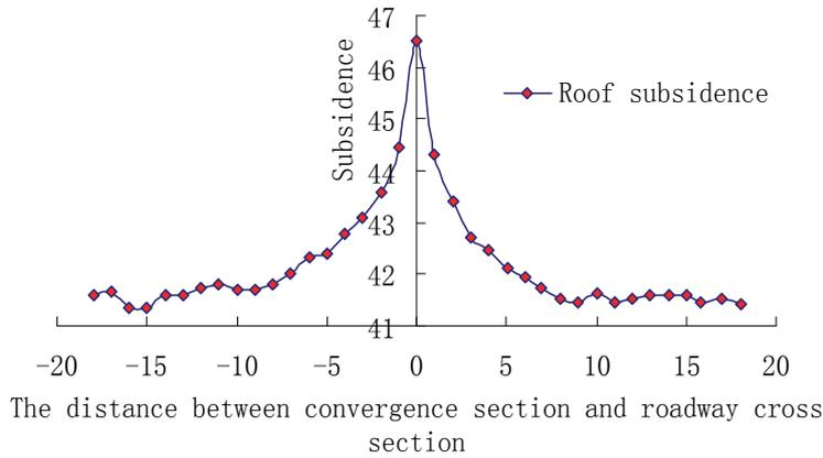
Figure 8 The main roadway vertical displacement curve
