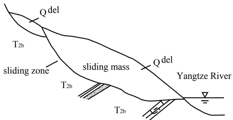
Figure 2 The geohydrologic unit of the Shiliushubao landslide
