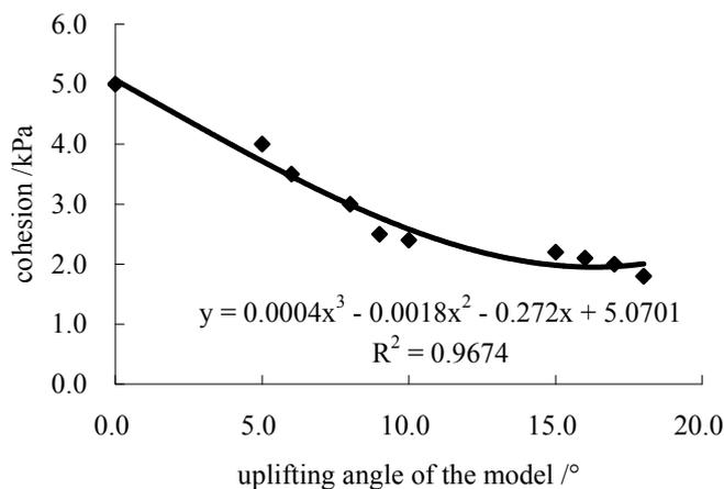
Figure 8 The curve of cohesion of sliding zone vs. uplifting angle of the physical model
