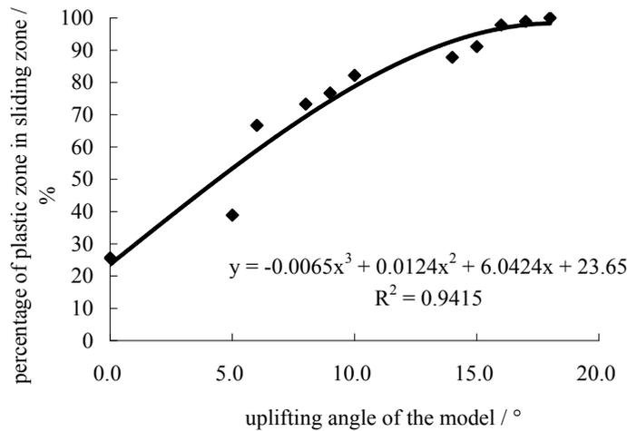
Figure 7 The curve of the percentage of plastic zone vs. uplifting angle
