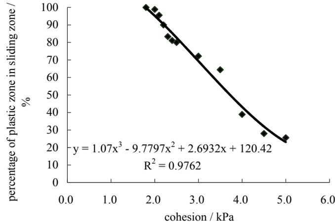
Figure 5 The curve of the percentage of plastic zone vs. cohesion of sliding zone
