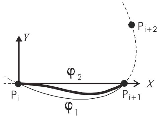
Figure 5 Straight to curve interpolation
