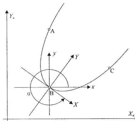
Figure 2 An oblique axis parabolic curve
