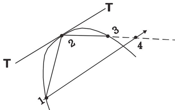
**Figure 12 Analytical method of determining the true azimuthal angle of oblique axis parabola**
