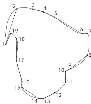
(a) Result of the oblique axis parabolic interpolation for curve smoothing
